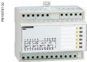
M6C programmable contacts: circuit-breaker external relay with six independent changeover contacts controlled from the circuit breaker via a three-wire connection. (maximum length is 10 meters).
